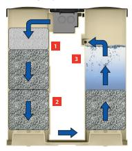
Oily water flows through pre-filter removing contaminents
